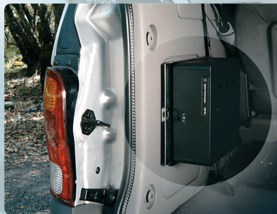
The Air Interface RMS probe mounts securely in any vehicle.
